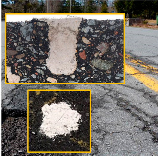
Researchers are trying to devise a better, cheaper way to fill potholes by combining solids from wastewater with calcium oxide, magnesium oxide, and a weak acid to make a cement-like binder. Image credit: Zhongzhe Liu (California State University, Bakersfield, CA).
